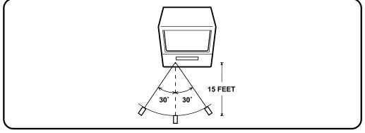
**NOTE:** • When there is an obstacle between the TV/VCR and the transmitter, the transmitter may not operate.
